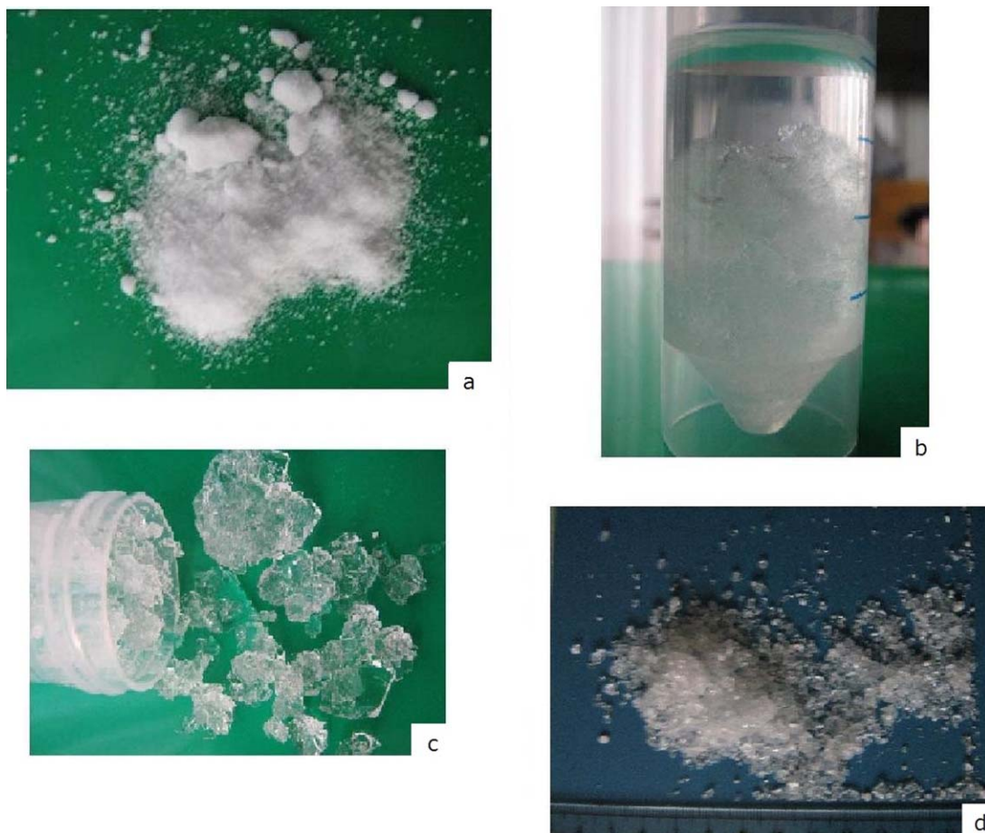
Figure 1. (a) TME powder, (b) Generation of TME · 3H 2 O crystal masses by addition of water to TME powder, (c) Dried TME · 3H 2 O crystal masses.
